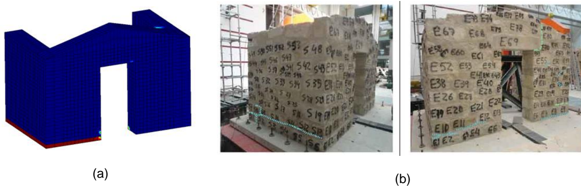
Figure 5.28 Stone house: (a) Numerical failure at the base of the south wall and (b) experimental early failure at the base of the south wall
