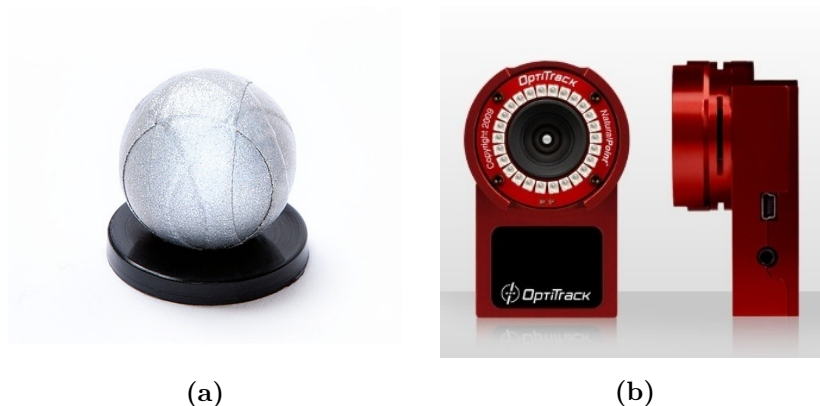
Figure 4.1 Reflective marker (4.1a) and model of camera (4.1b) used for the motion capture.
