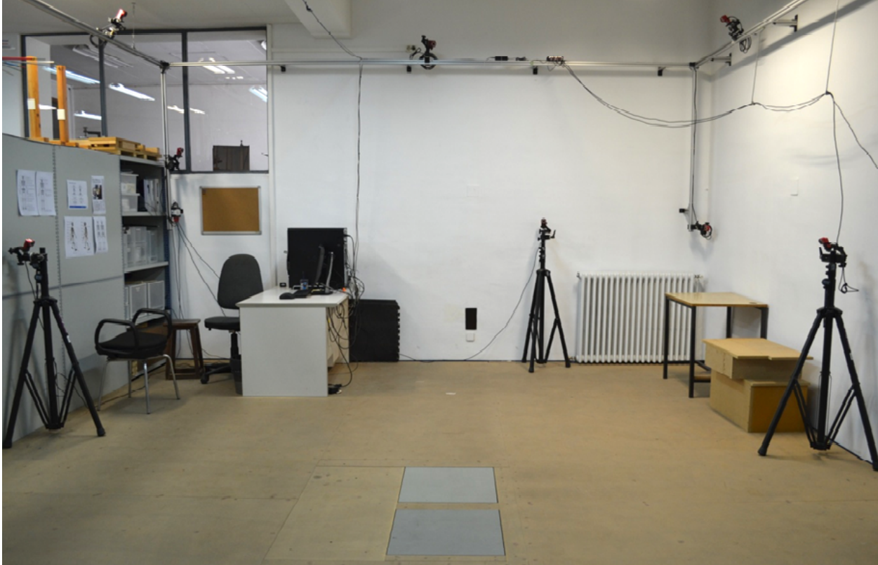
Figure 4.2 View of the Biomechanics Lab. Cameras can be seen in high and low position, as well as two force plates at the center of the room.
