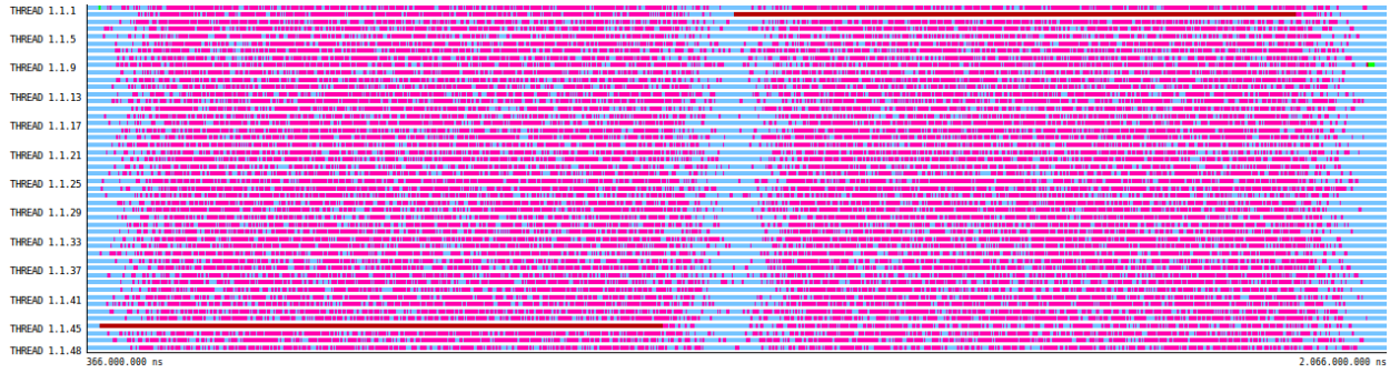
Figure 7.22: Coarse grain N-Body execution trace on ThunderX with 48 threads and Nanos++
