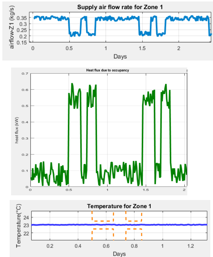
Fig. 8.8 Effect of occupancy on temperature and supply air flow in one zone
