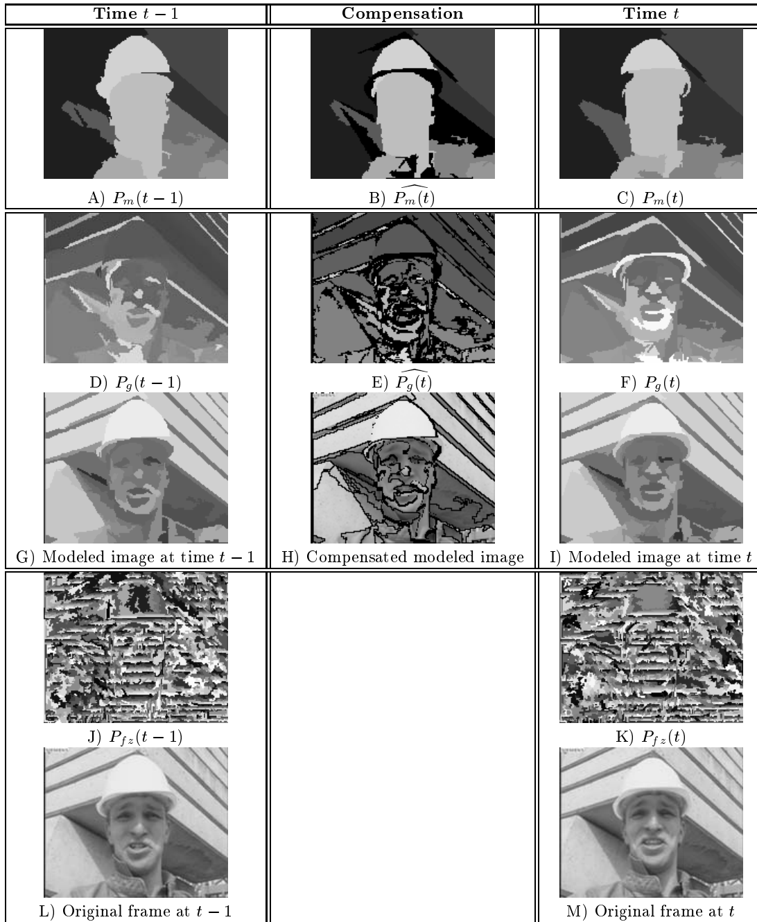
Figure 11: Example of gray level sequence segmentation: first column: partitions and frames at time t - 1 , second column: compensated information, third column: partition and frames at time t . Partitions are represented with their label to see the region tracking ability of the algorithm.
