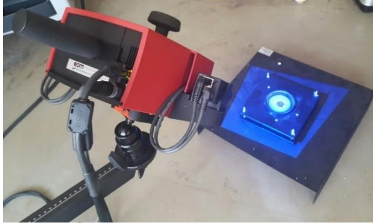
Fig. 4 The ATOS-3D scanner adopted for the optical measurements of the specimens
