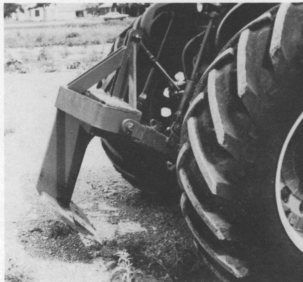
Front-end and rear-end mounted tree grubbers are most effective for control of small mesquite trees and sprouts.
