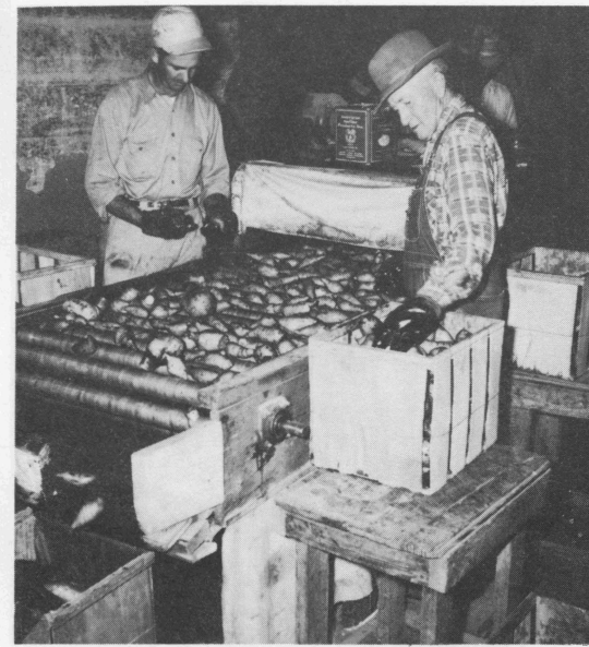
A roller conveyor on which sweet potatoes are washed, waxed, sorted and graded. Less bruising results when sweet potatoes are placed in the crates by hand.
