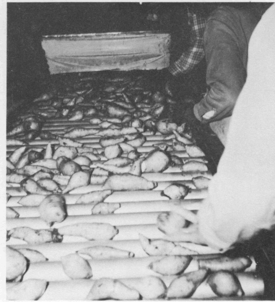
A roller conveyor on which sweet potatoes are washed, waxed, sorted and graded. Less bruising results when sweet potatoes are placed in the crates by hand.
