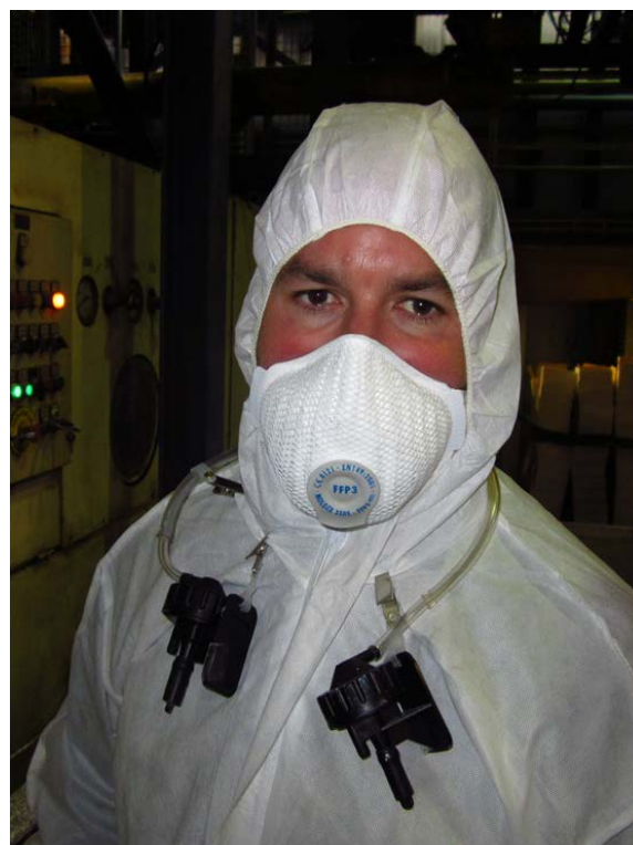
Figure 4. Picture taken during a break period in the manufacturing activities, showing a worker carrying two personal samplers (cyclones) for the capture of the aerosol respirable fraction, addressed to off-line analysis (gravimetric, chemical and microscopic).
