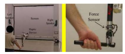
Fig. 2. On the left, the experimental setup comprising of a projector screen, the six-DOF LHIfAM haptic device and a pair of speakers. On the right, users hold the LHIfAM's stylus in the form of force grip.
