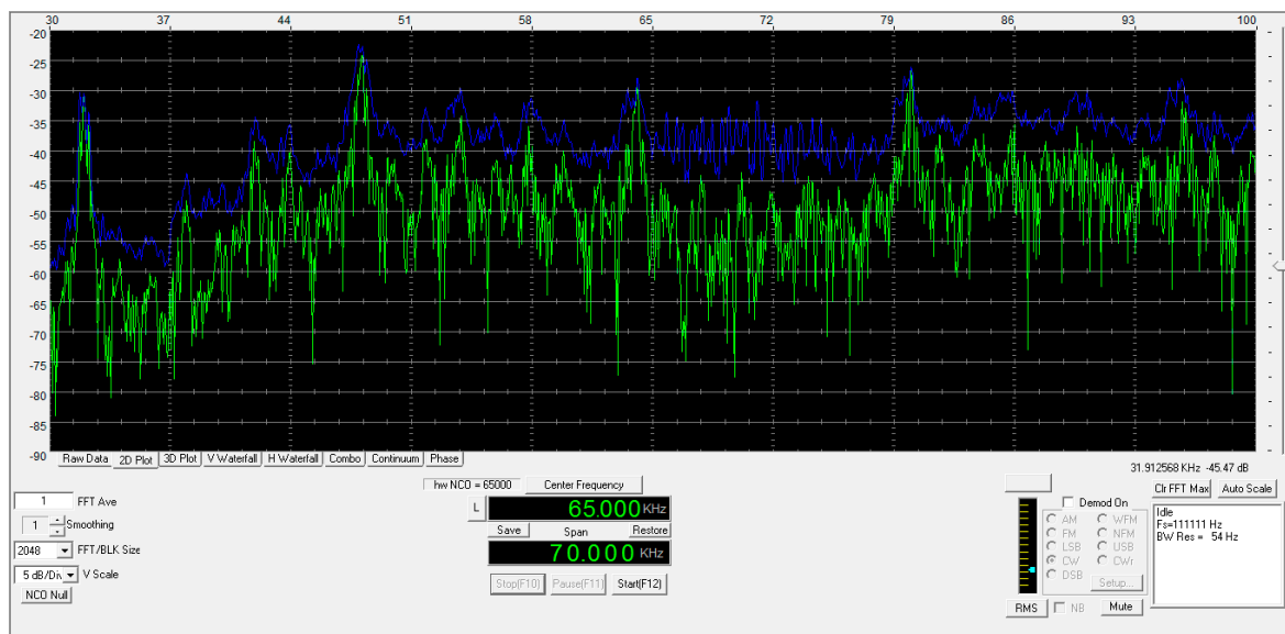
Figure 17. Noise associated to the inverters.
