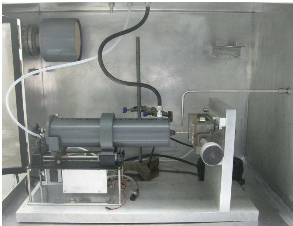
Figure 2: Apparatus setup of drilling within enclosed chamber with front window panel removed and side door open
