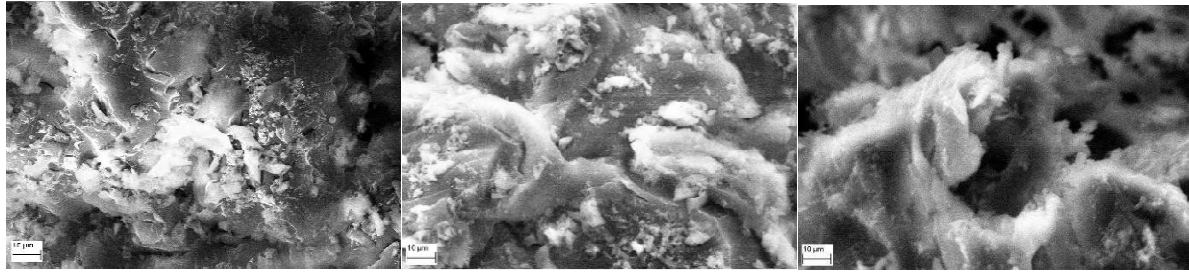
Figure 9: SEM images of collected debris from sampling tray within chamber of Neat Epoxy (left), EP/CNF (middle) and EP/CNT (right) samples
