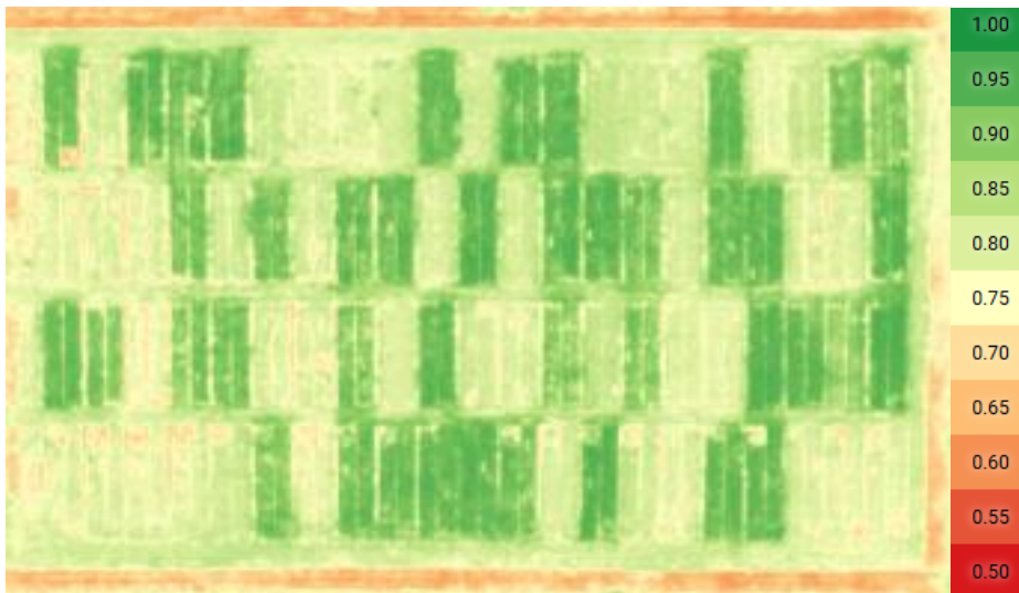
Figure A-2. Aerial photo taken by a MicaSense RedEdge camera mounted on a UAV drone to measure normalized difference vegetation index. Higher NDVI values in experimental units that received foliar fungicide (green rectangles and Treatment 6&8), and no foliar fungicide resulted in lower NDVI values (Treatment 1&13) at Belleville 2016-17 on June 7, 2017.
