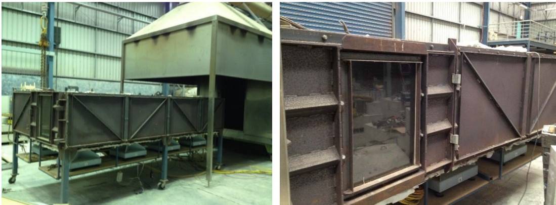
Figure 5. The experimental rig after modification of the original enclosure (window locations included). The dimensions of the modified enclosure was 4 m long (D), 2 m width (W) and 0.6 m high (H). One side (2.0 m × 0.6 m) of the enclosure was fully opened for ventilation. All other sides were closed by the steel walls. There were also two glass windows on the enclosure wall which were used for observation of the fire behavior in the rig. The windows were constructed from fire-resistant glass and one was placed at the back side of the enclosure while the other was on one of the side walls and close to the opening side. The geometry of the enclosure and location of the windows are shown in Figure 5.
