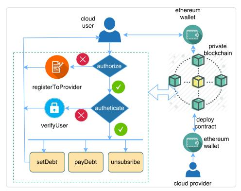
Figure 10: Prototype: Flow diagram
