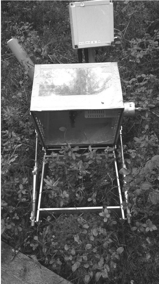
Fig. 1. Automated measurement chamber used in this study. The chamber sits in an aluminium frame, which is pushed into the litter layer and anchored to the soil.
