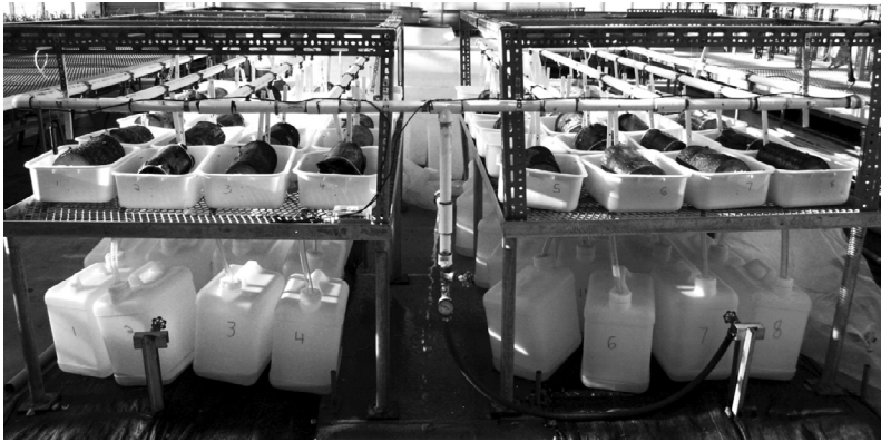
Fig. 1. Photograph of the greenhouse experiment setup showing the suspended logs, overhead misting nozzles, and collection containers.
