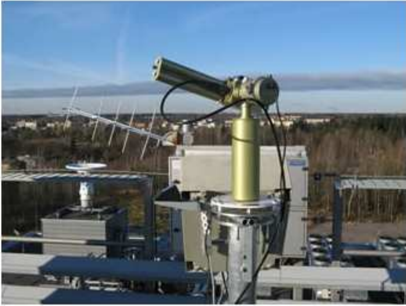
Figure 8: The sun photometer measuring on the roof of Finnish Meteorological Institute main building, Helsinki, Finland.
