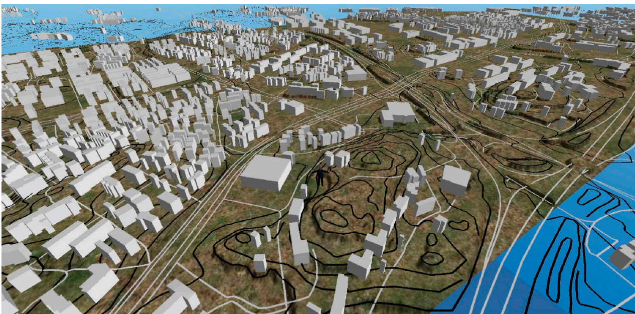
Figure 5. Buildings, roads, terrain, and contours in Meshmoon in an early, manually created version.
