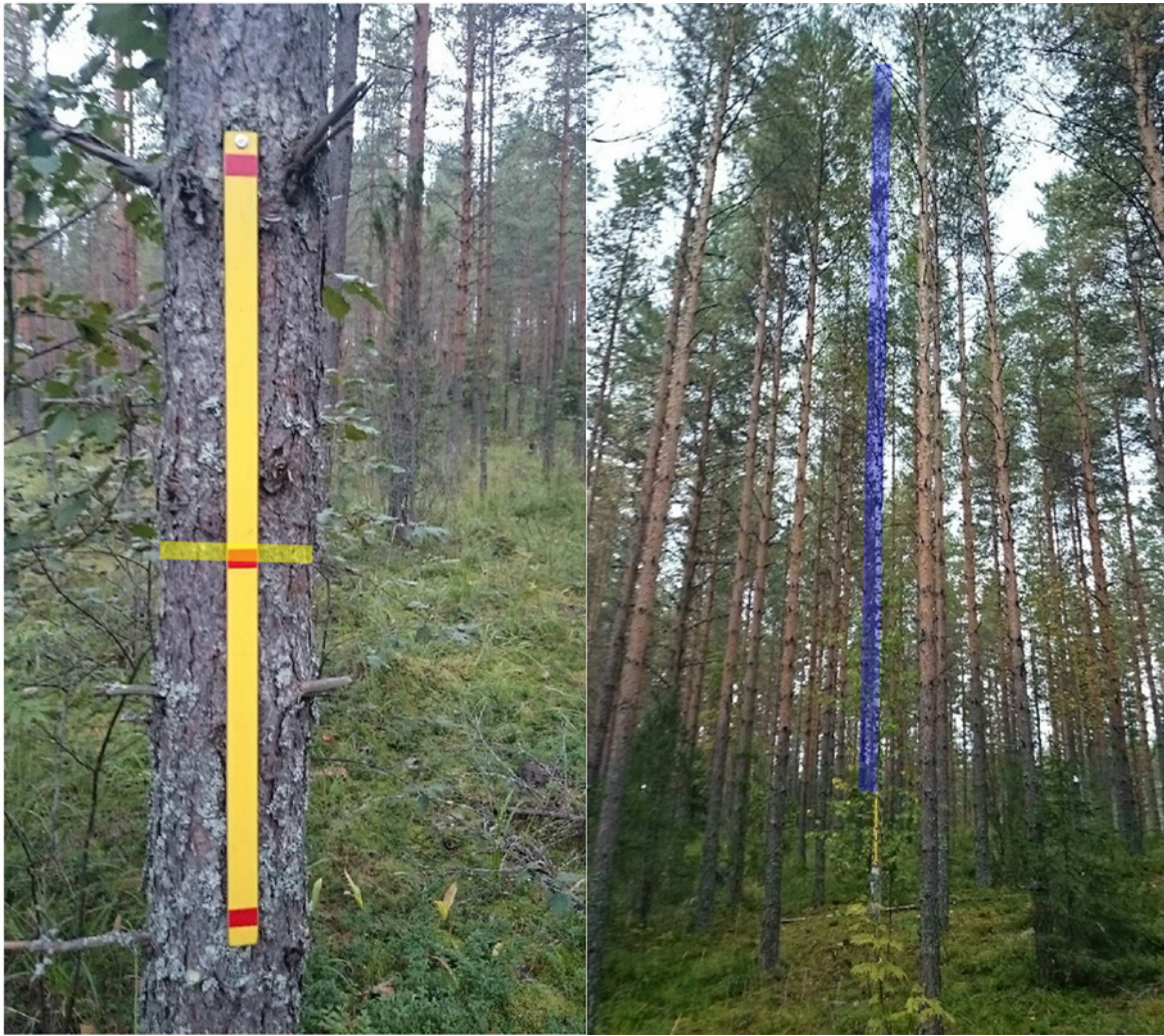
Figure 3. Measurement stick (1 m in length) is required to scale the image and measure dbh and height of the median trees.
