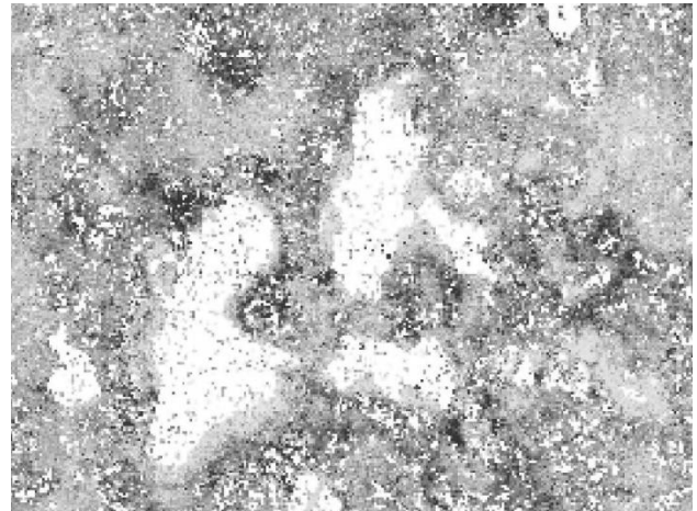
Figure 5. Canopy height model (10 m resolution) derived using radargrammetry.
