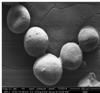
Fig. 1 SEM image of CS-CPP modified nanoparticles encapsulated in the HPMC-AS polymer (H-PLGA particles).
