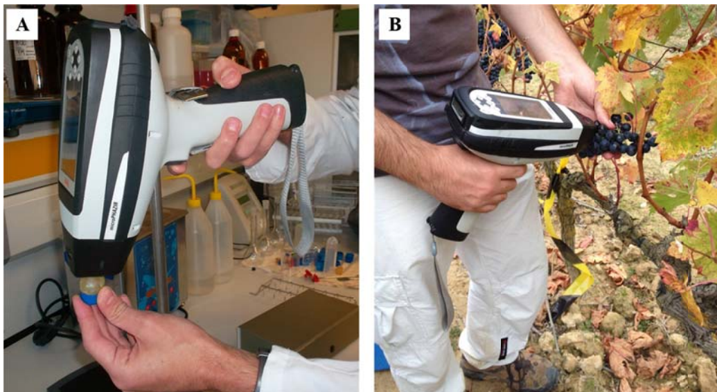
Figure 1. Spectra acquisition in (A) laboratory, and field conditions (B) using the portable microPHAZIR™ (ThermoScientific, Waltham, MA, USA) NIR spectral analyzer, used for non-invasive assessment of total soluble solids.
