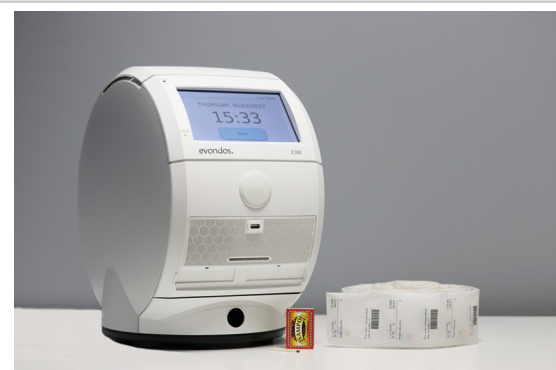
Figure 1. Evondos E300 Medicine Dispensing Robot with Multidose Sachets (Salo, Finland). The matchbox is included to indicate relative size. It measures 2.2 inches in height and 1.4 inches in width.
