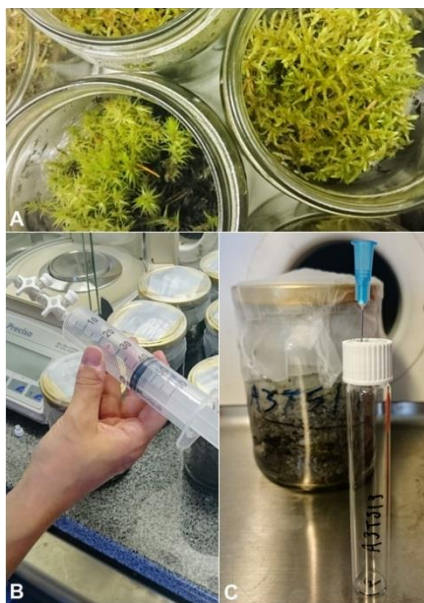
Figure 3. ARA experiment. A: Moss samples. B: Addition of acetylene before incubation. C: Gas transfer to vial after incubation.
