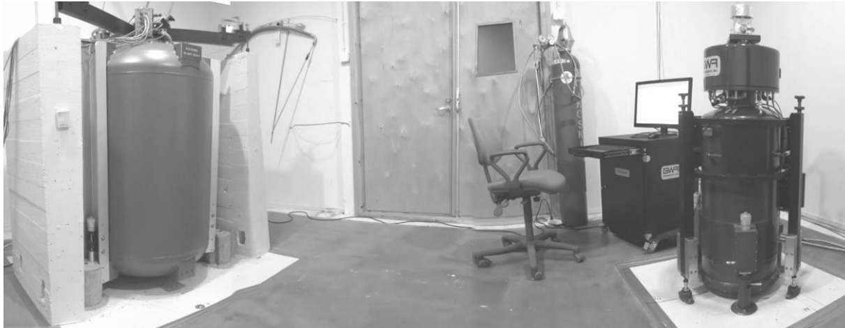
Figure 1. Superconducting gravimeters at Metsähovi. The old T020 on the left and the new OSG-073 on the right.
