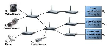
Fig. 1: An example WSN network with missions of different priorities, consuming data from multiple shared sensors.
