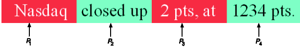
Fig.2. Original image. It includes four tiles. The codestream of each tile is encapsulated into one IP packet.
