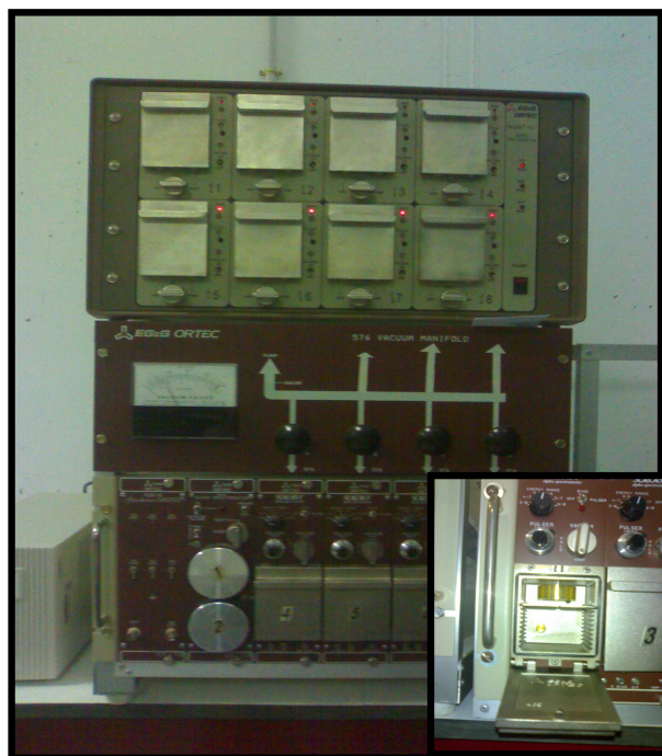
Fig. 3. Picture of measurement system at the Radiochemistry laboratory at the University of Huelva. In the inset, the detector and the sample holder can be seen.
