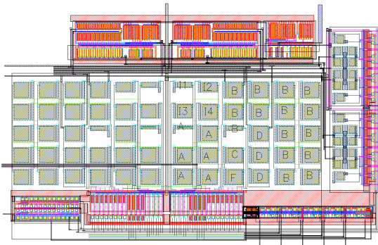
Fig. 9 Layout view of the sinusoidal generator with harmonic cancellation
