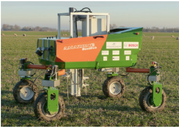
Figure 3. Bonirob with a soil penetrometer
