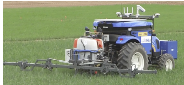
Figure 7. Herbicide application using intelligent boom spray in a wheat field
