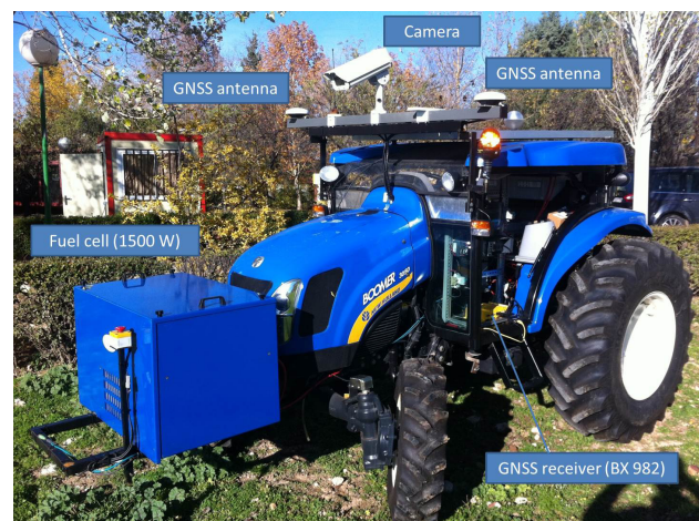
Figure 6. Modified New Holland Boomer T3050
