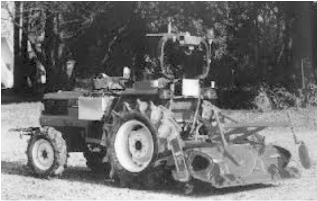
Figure 2. Robotra performing a tilling operation
