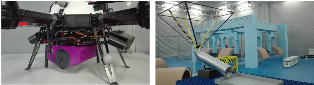
Figure 6.12: Small cargo bay on the UAV (left) and hopper for autonomous delivery (right).
