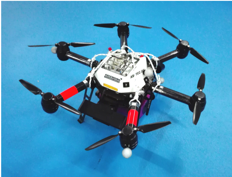
Figure 3.17: The UAV with the RGB-D sensor at the front.
