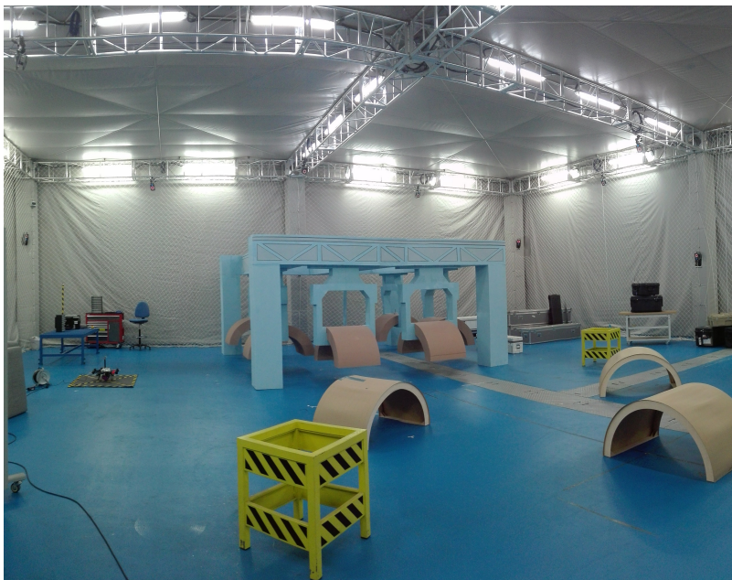
Figure 5.3: The indoor testbed at CATEC with a mock-up scenario for 3D map building.
