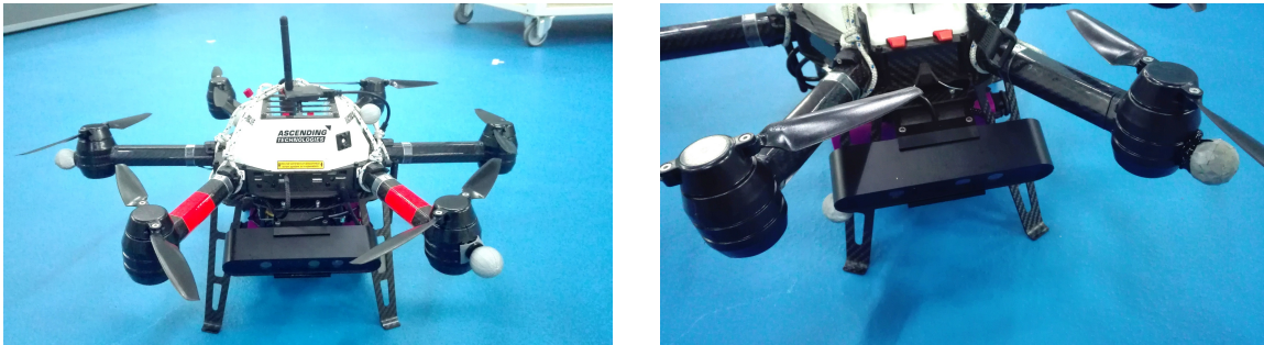
Figure 5.2: The UAV with RGB-D sensors at the front (left) and the rear (right) side, and a UWB sensor on top.
