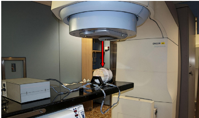
FIG. 1. Experimental setup showing the accelerator's head where the collimating system is installed, and the cylindrical phantom described in Sec. II. The arrow shows the direction of the beam.
