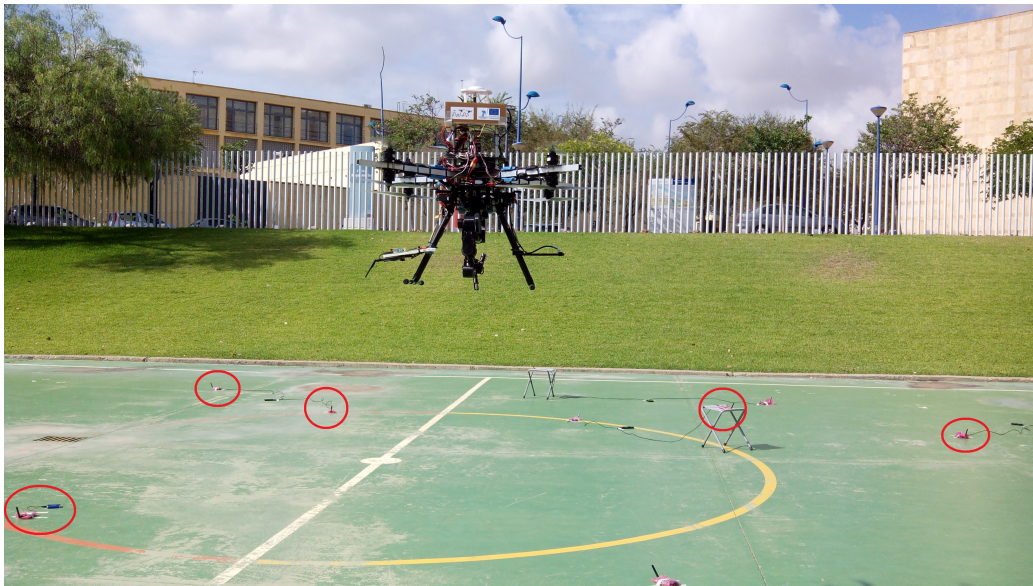
Figure 7.3: AMUSE UAS flying during one experiment at the School of Engineering of Seville. Beacons are marked with red circles.
