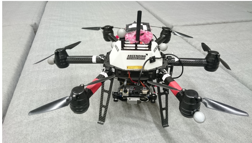
Figure 7.2: AscTec Neo with a Nanotron range sensor.
