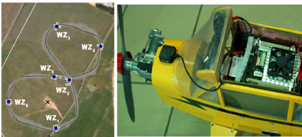
Figure 9. (Left) Estimated flight plan and actual UAV trajectory (black line) obtained in field experiments. (Right) Picture of the embedded PC104 in one Piper airframe used in the experiments.
