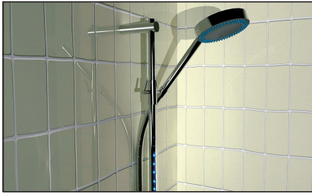
Figure 1. The shower prototype. An ambient display can help people by giving immediate and direct feedback regarding water consumption.
