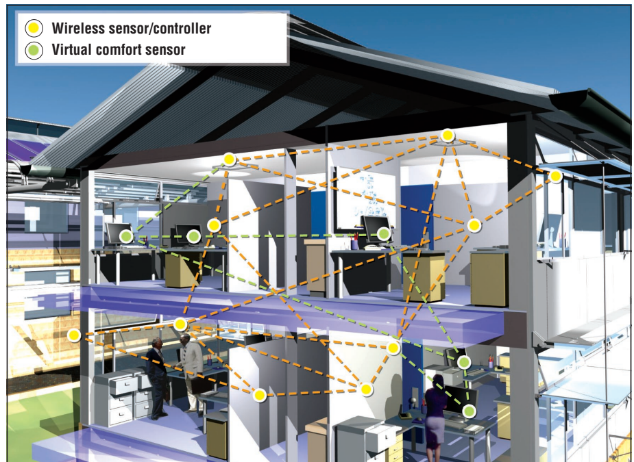
Figure 4. Integration of wireless sensors/controllers and virtual comfort sensors for optimal, distributed control of sustainable buildings.
