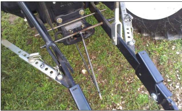
Figure 4. Implemented steel tillage bar on the autonomous tractor.
