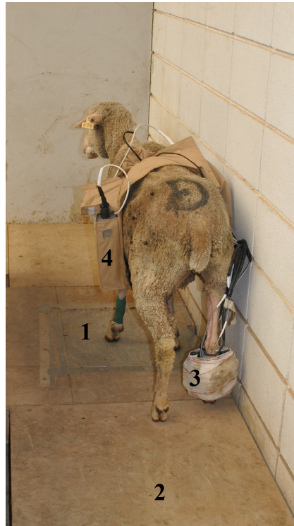
Figure 3.10: Sheep during a gait test [115]: (1) force platform; (2) wooden platform; (3) instrumented fixator; (4) A/D converter for the load cells signals.
