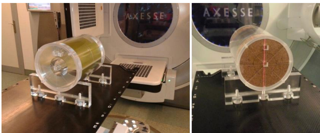
Figure 3.17. Final PMMA phantom QuAArC with rolled radiochromic EBT3 films (left) and PMMA slices for axial films with cork cylinders (right).
