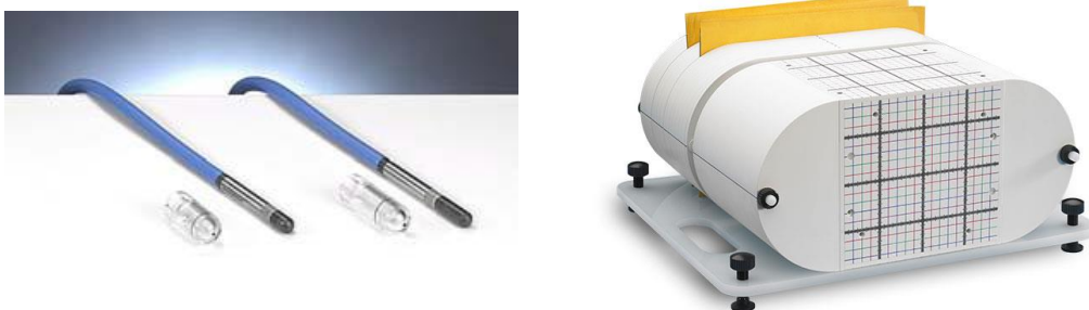
Figure 1.3. PTW Semiflex 0.125 cm 3 and 0.3 cm 3 ionization chambers (left) (PTW), and films placed in the Easy Cube phantom (right) (DonaldsonMarphil).
