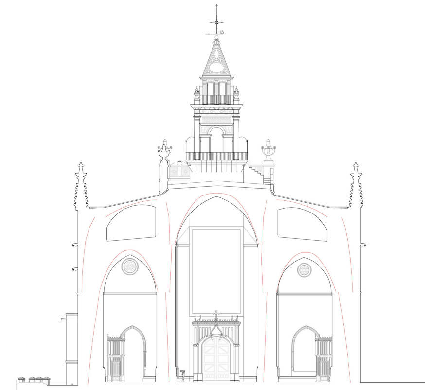
Figure 7. Thrust line analysis of the transversal section including columns number 2 (right) and 6 (left).
