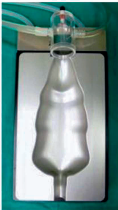
Picture 3. Self-designed, adjustable water heating tub for heat supply in guinea pigs during surgery. Aluminium surface and a notch for the nose cone.
