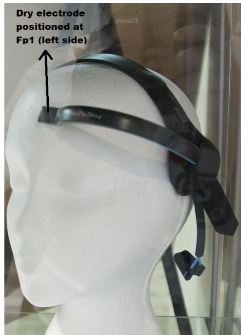
Figure 2.5. Neurosky mindwave mobile headset 21 . The electrode is positioned in the left side of the forehead.
