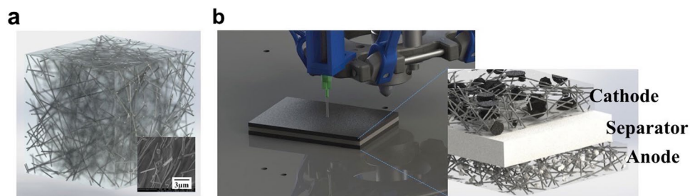
Figure 1. Schematic designs of cellulose composite and 3D printing of battery composites. (a) Computer aided design (CAD) model of AgNW/CMC 3D Conductor. Inset shows the scanning electron microscopy (SEM) image of the AgNW/CMC 3D Conductor, (b) CAD representation of three-layered 3D printed battery.
