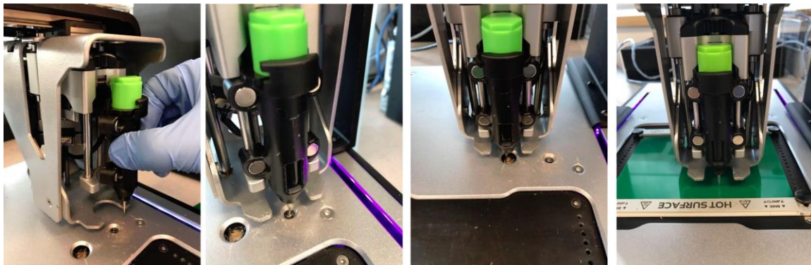
Figure 3.5. Calibration procedures for substrate height profile
