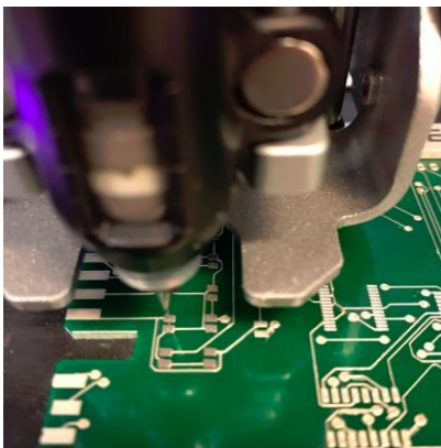
Figure 3.13. Image of dispensed solder paste on printed circuit pads
