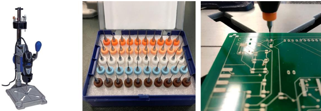
Figure 3.9. (left) Dermer Mode 3000 press driller (middle) PCB drill bits set (right) image of drilling process for through-hole and vias
