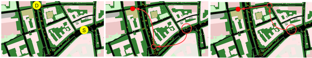
■ Figure 1 Motivating example to dynamic self-organizing routing. Whereas a car may take the apparently optimal route from S to D (middle) it may also avoid causing unnecessary congestion and use the route depicted to the right. Best viewed in color.
