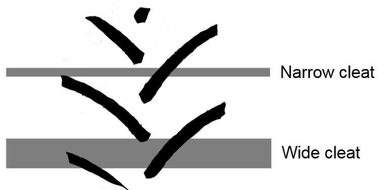
Figure 40: Tread pattern of a tractor tire passing two different cleat width
