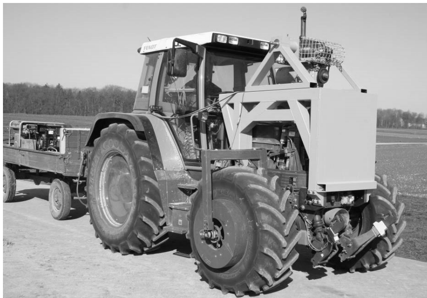
Figure 38: Shaker installed on Fendt Favorit 509
