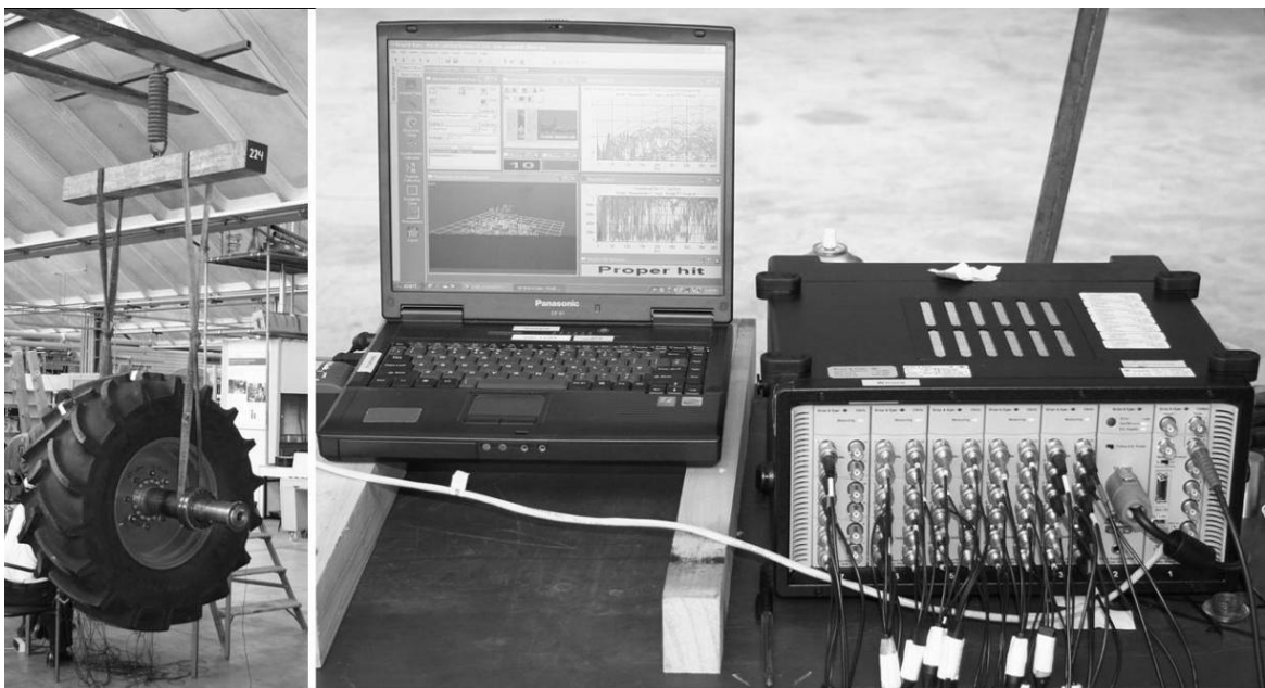
Figure 17: Measuring setup for Experimental Modal Analysis
