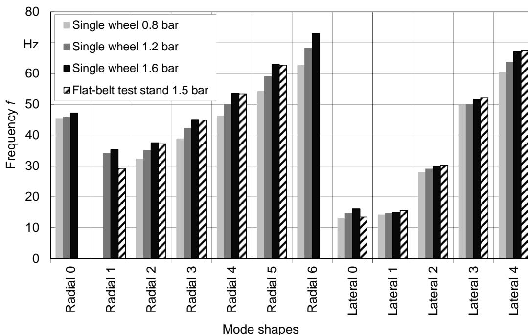
Figure 69: Eigenfrequencies of an unloaded Goodyear Optitrac 520/70 R38 (Rear) mounted in the test rig ( p_i = 1.5 bar) compared with results of modal analysis of the single wheel (5.1.1) ( p_i = 0.8 / 1.2 / 1.6 bar)
