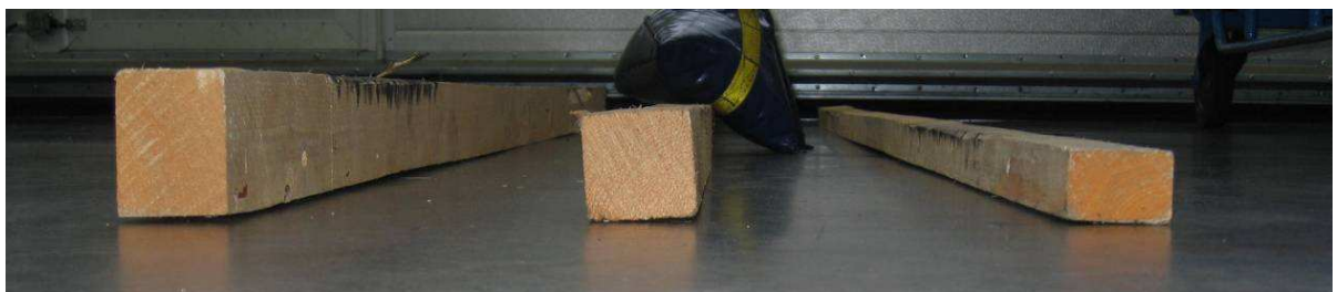
Figure 41: Wooden cleats, height: 78/58/38 mm, width: 58 mm
