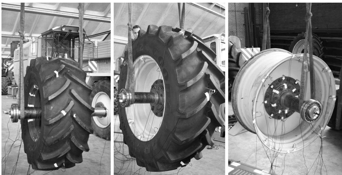
Figure 20: Suspended wheels and single rim
