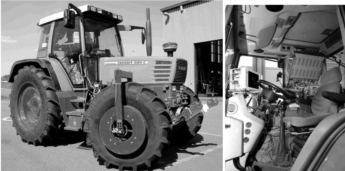
Figure 33: Instrumented Fendt Favorit 509 C with view inside the cabin
