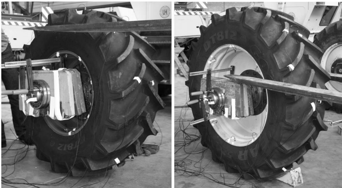
Figure 21: Loaded wheel assembly
