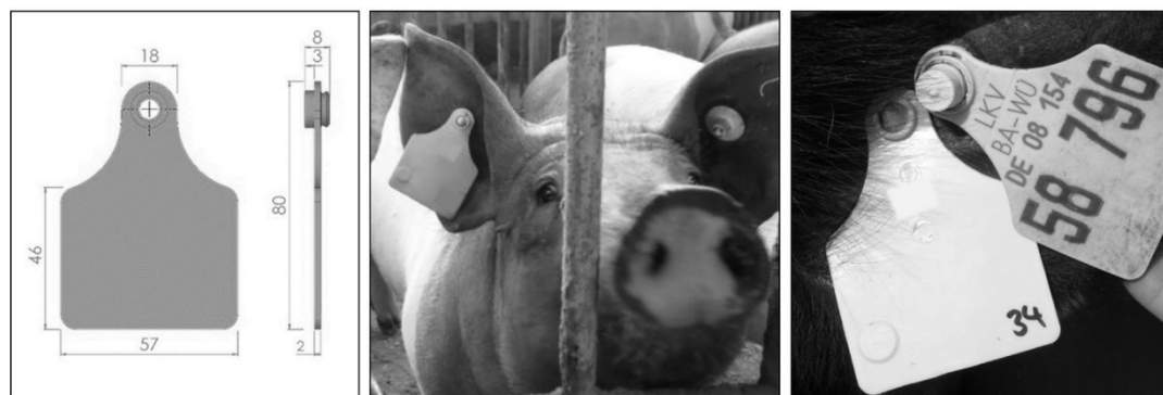
Fig. 1. Dimensions (mm) of the Primaflex ® ear tag (left), pig with UHF transponder ear tag in its right ear (centre) and cattle ear with UHF transponder ear tag (ear tag 34) and standard visual ear tag (right).
