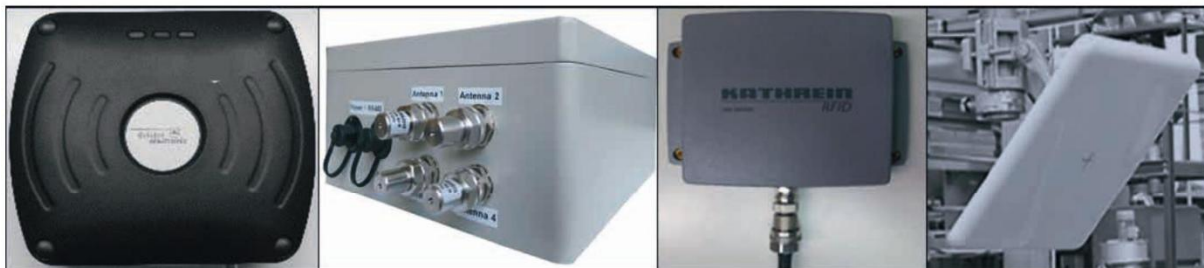
Figure 2: Reader TSU 200 with integrated antenna, TSU 200 Mux with four external antennae connections, external antenna from Kathrein-RFID, "Mira 52010082" and external antenna from MTI, "Antu-Patch 63" (l to r) (© F. Adrion)
