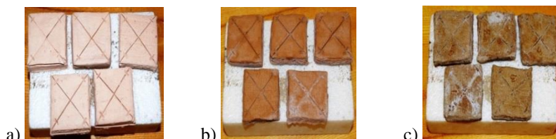
Figure 1 - Samples after sintering: a) kaolin; b) loam; c) red clay.
