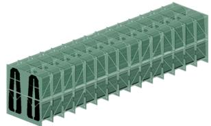
Fig. 1. The module of tube bundle of condenser.
