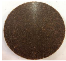
Fig. 4. Preform from bran and shell of cedar nuts, got pressing at 150°C.
